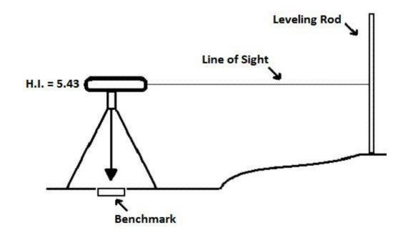
In the drawing shown, the survey instrument reads 4.17 on the leveling rod. The height of the instrument is 5.43. The benchmark elevation is 214.56.
